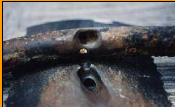
Pit Corrosion in a gas line
